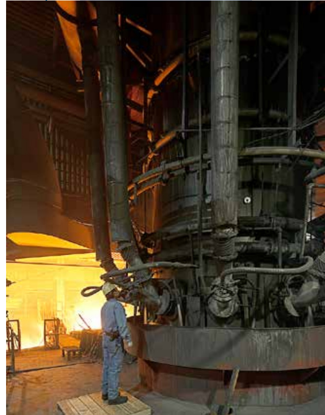
A Waupaca Foundry melt operator checks the cupola tuyeres at its Tell City, Ind., foundry.
